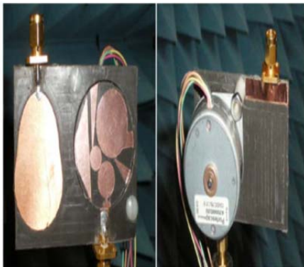
Figure 19: Mechanically reconfigurable antenna (Image Source: [31])
